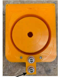
Figure 1. Tab to be inserted in a vice for hand cutting
