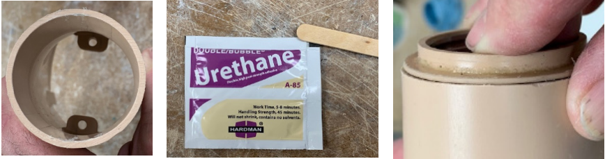
Figure 9. You should not see the O-ring when fully seated and glued in place.
