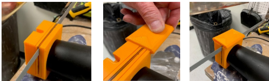
Figure 6. Cut through guide slot with a hack saw.
